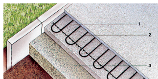
1 = béton 2 = tapis chauffant 3 = support
